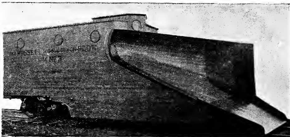
Fig. 224. THE RUSSELL DOUBLE TRACK SNOW PLOW. (The framing is shown in Fig. 409.) Snow Plows built by The Ensign Manufacturing Company.
